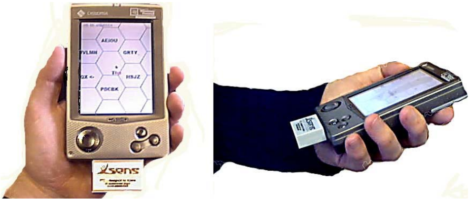
Fig. 4. The system running on Cassiopeia E115 with a miniature accelerometer
